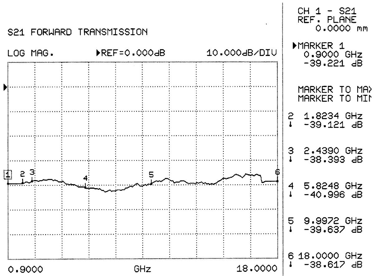
Device under test #2: **RF- and Microwave Shielding Paint HSF54**
