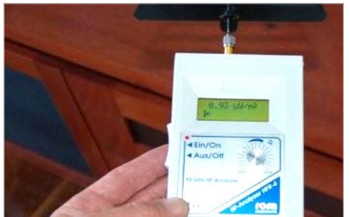
10) Excellent low reading of 0.93 microwatts per metre squared after shielding.
