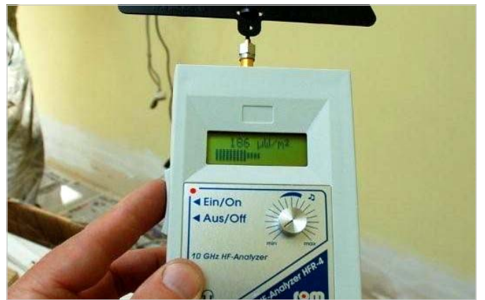
4) High reading of 186 microwatts per metre squared pre shielding.
