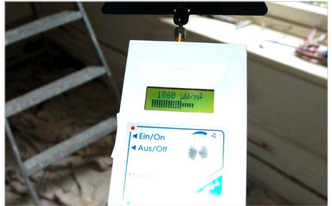
2) Very high EMR reading of 1860 microwatts per metre squared prior to shielding.
