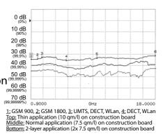
underground / the substrate of the shielding paint coat. Due to this new development no ground strap is needed for safe grounding of the shielding paint coat, specifically in outdoor applications. • Can easily be covered with two top layers of water based emulsion paint. • **The paint is frost resistant** (tested for 5 freeze / thaw cycles).
